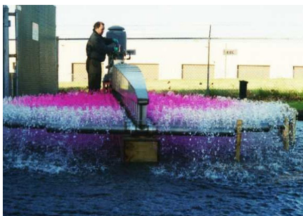
Johnson Screens has patented an advanced collector distributor system design that allows for fractal control of fluid flow in a media. This flow is demonstrated by the even distribution of the dye through the water.
